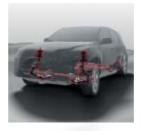
**Kinetic Dynamic Suspension** System (KDSS) Off-road Drive off-road and the wheels remain firmly on the ground and provide greater traction. The stabiliser is disconnected. With the fluid now allowed to flow freely through the system, each wheel can move with much more independence on uneven ground. The resulting longer wheel travel provides uncompromised traction and stability on the roughest terrain.
